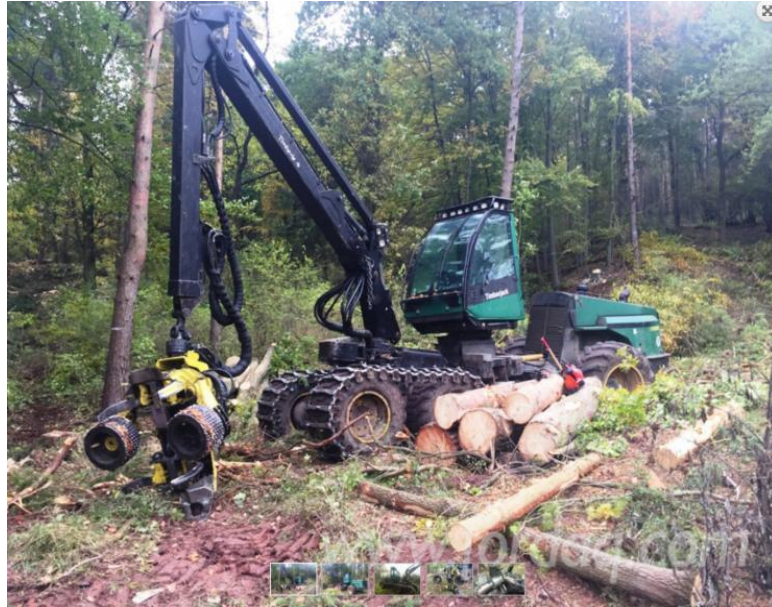
Slika 5. Harvester, Timberjack 1470D
