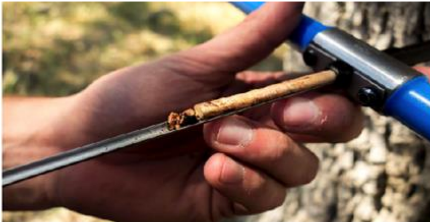
Slika 1. Pressler-ovo svrdlo (eng. increment borer) ( https://www.skepticalscience.com/print.php?n=2774 )
