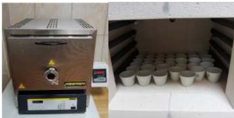
Slika 19: Mufolna peć Nabertherm L9/13/B180
