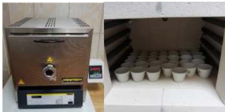
Slika 19: Mufolna peć Nabertherm L9/13/B180
