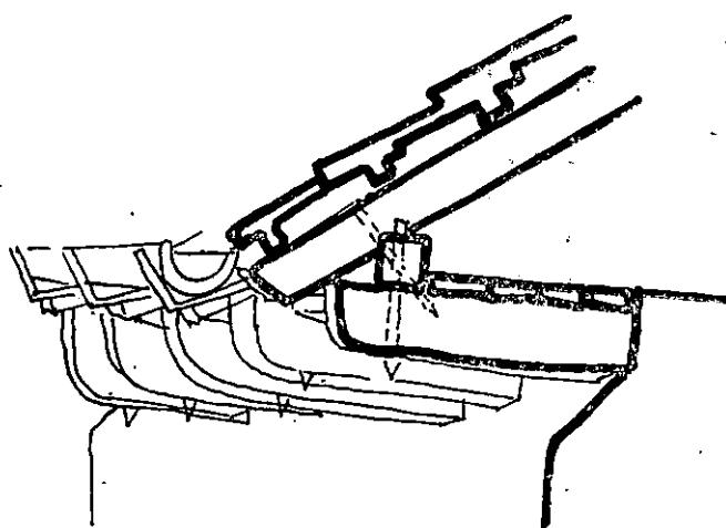
Sl. — Fig. 11. Detalj krovne konstrukcije sa strehom i žlijebom — A detail of a roof construction showing eaves and gutter.
