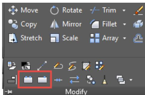
Slika 7.142 Odabir alata *Break* i *Break at Point*
