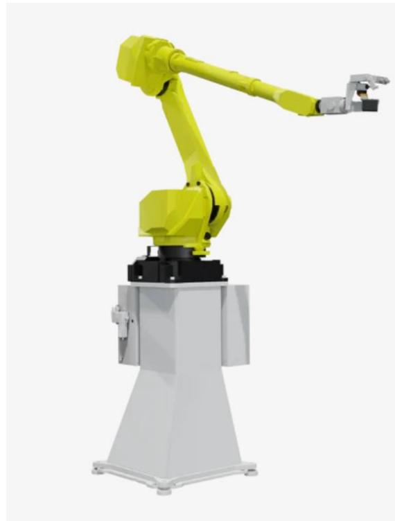
Slika 13 Robot za štrcanje ([www.ceflafinishing.com](http://www.ceflafinishing.com))
