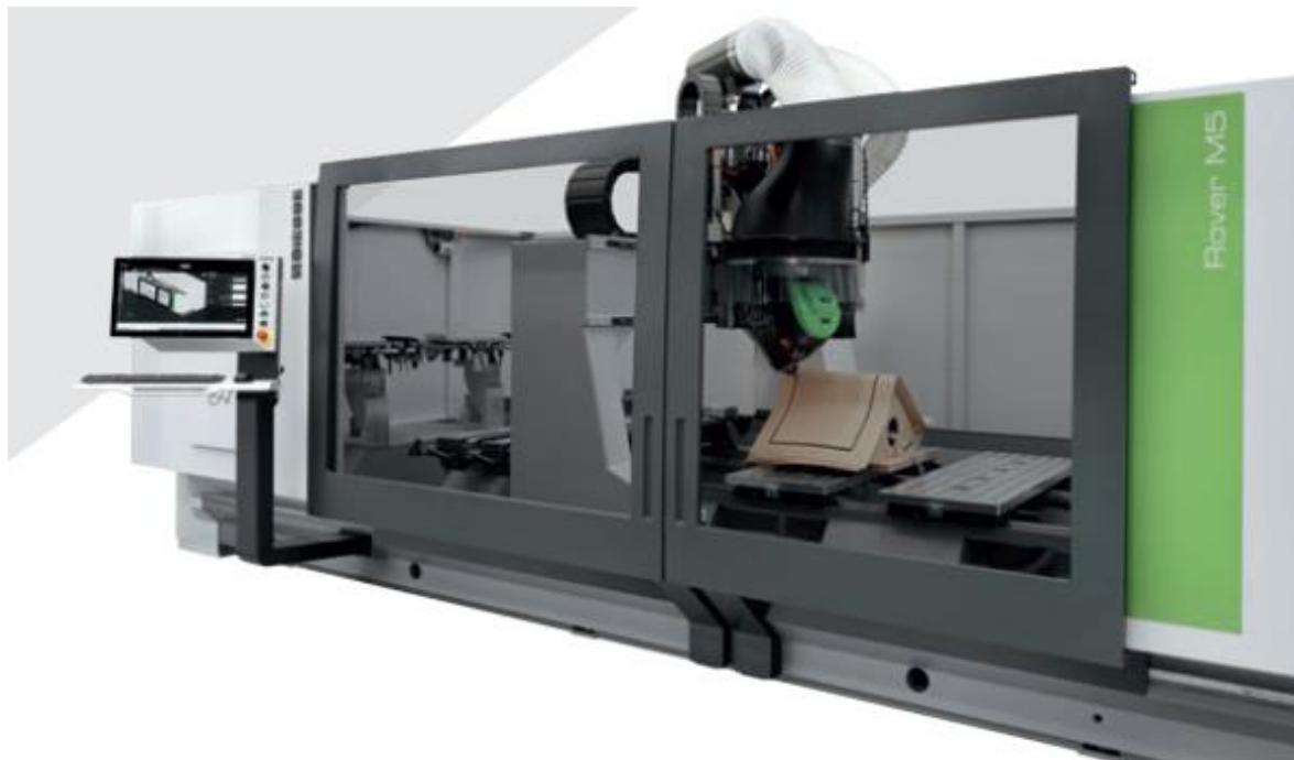
Slika 8. Biesse Rover M5 prikazan u zahvatu složenog obratka velike visine ([http://www.biesse.com/ww/biesse\\_products/rover/rover\\_m5](http://www.biesse.com/ww/biesse_products/rover/rover_m5))
