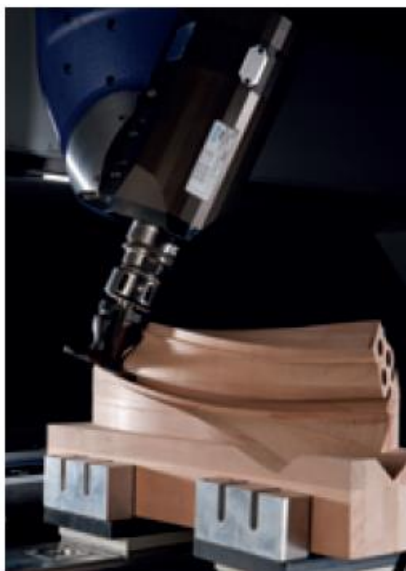
Slika 5. Homag DRIVE5C+ 5-osna radna glava ( https://www.homag.com/en/product-detail/bmg-500600_processing-centers/ )
