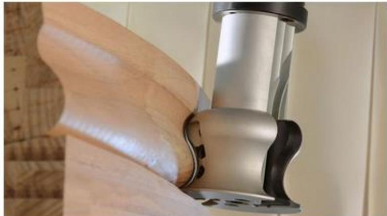
Slika 14. Prikaz obrade masiva velike visine profilnim glodalom na HOLZ-HER Pro Master 7225 CNC stroju (<https://www.weiniq.com/en/panel-processing/cnc-machining-centers/pro-master-72-series.html> )
