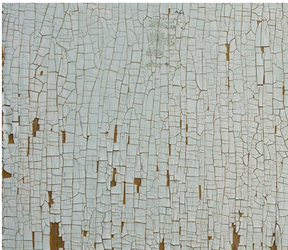
Slika 4. Krokodilska koža ( https://www.ppgpaints.com/pro/pro-painting-tips/how-to-fix-alligatoring-with-paint )
