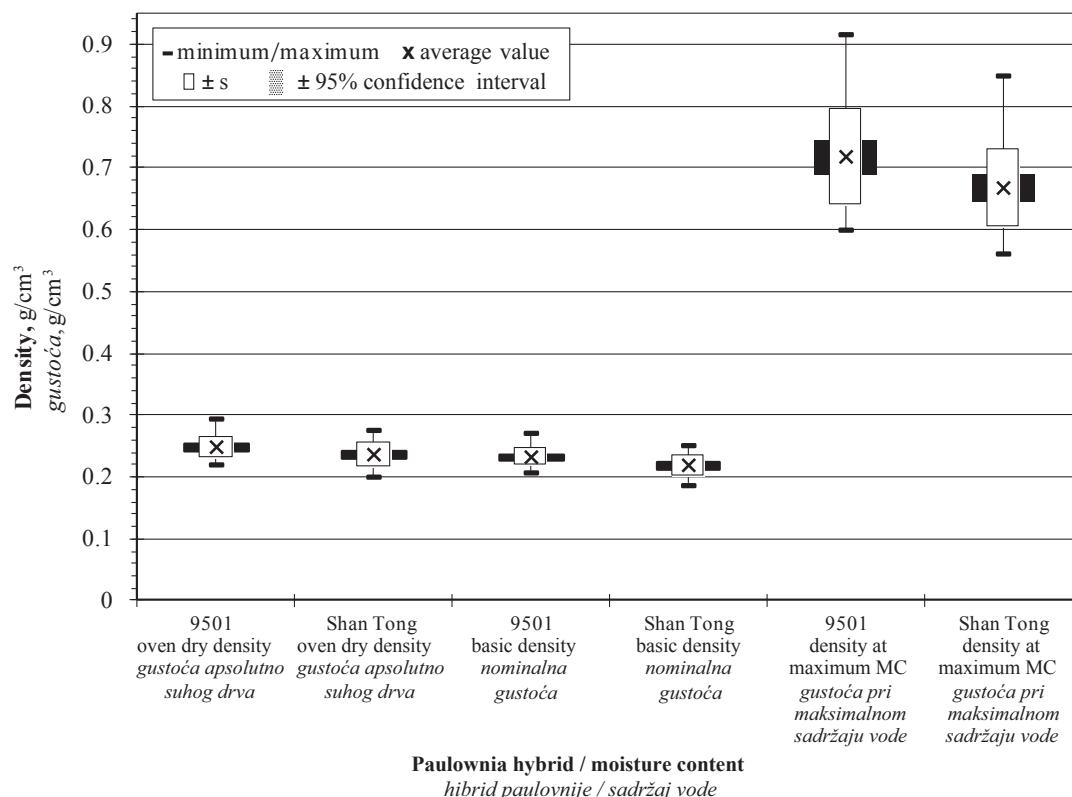
**Figure 2** Statistical analyses of oven dry density, basic density and density at maximum MC, between two paulownia hybrids
