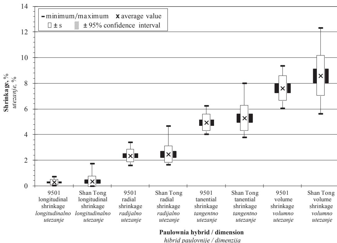
**Figure 1** Statistical analyses of longitudinal, radial, tangential and volume shrinkage, between two paulownia hybrids
