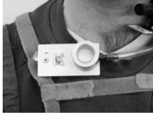
Fig. 2. Holders of filters sampling respirable particles (a) and total wood dust (b).
