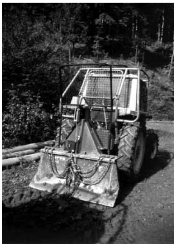
Slika 4. Traktor Steyr s jednobubanjnim vitlom Tajfun EGV 60A Figure 4 - Tractor Steyr with single drum Winch Tajfun EGV 60A
