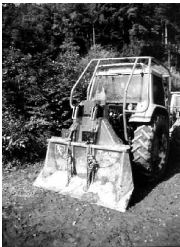
Slika 5. Traktor Steyr s dvobubanjским vitlom Tajfun 2 x 50 kN Figure 5 - Tractor Steyr with double drum Winch Tajfun 2 x 50 kN
