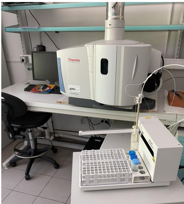
Slika 3. Instrument ICP-AES (Thermo Fisher iCAP6300 Duo)
