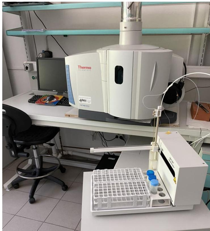
**Slika 3.** Instrument ICP-AES (Thermo Fisher iCAP6300 Duo)
