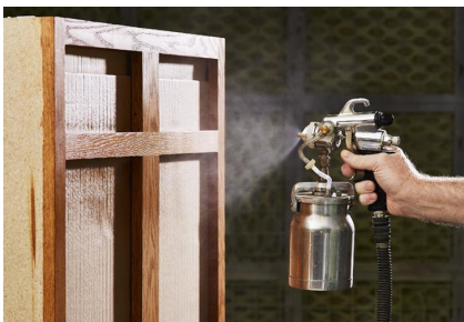
Slika 9. Prskanje s niskim tlakom (HVLP pištolj) ( https://www.woodmagazine.com/wood-supplies/finishes-finishing/spray-finishing-made-simple , pristupljeno: 24.8.2021.)
