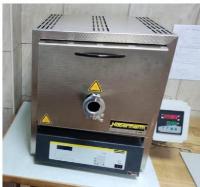
**Slika 17.** Mufolna peć (Nabertherm L9/13/B180)
