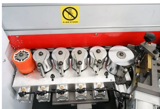
Slika 28. Primjer pritiskih valjaka (Izvor: Blue Elephant https://www.elephant-cnc.com/pro/e-70a-pneumatic-adjustment-automatic-edge-banding-machine-for-plywood-mdf-wood-furniture/ ; Pristupljeno 5.9.2022.)
