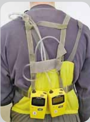
Uzorkovanje drvene prašine opremom B Collecting of wood dust samples using equipment B
