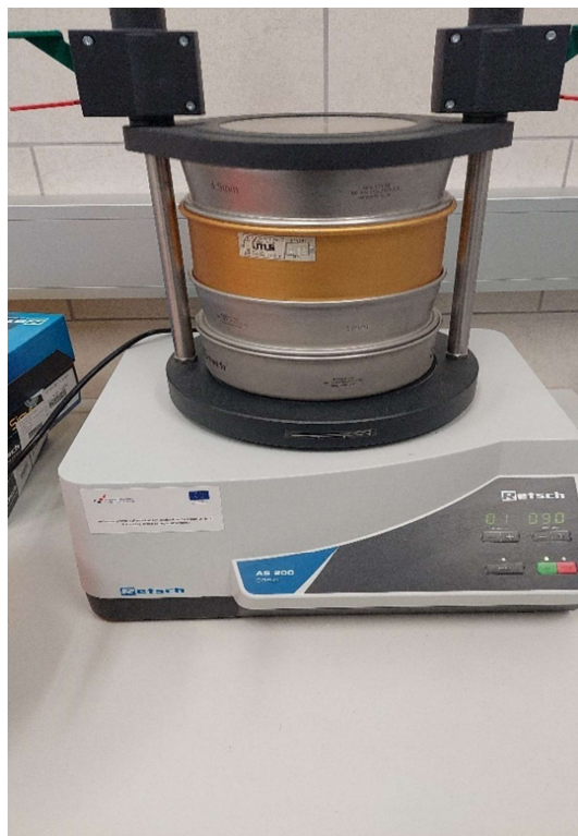
Slika 5. Tresilica sita Retsch AS 200
