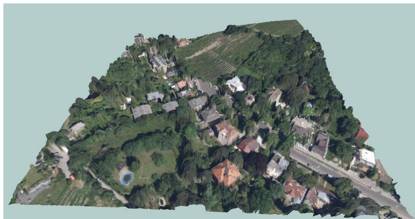
Slika 2. Ortofoto prevučeno preko digitalnog modela reljefa ( https://www.researchgate.net/figure/Example-of-a-3-dimensional-terrain-tile-from-an-orthophoto-and-a-DSM-Cobenzlgasse_fig2_342611763 )
