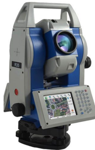
Slika 7. Totalna stanica Stonex R35 ( https://stonex.hr/product/r35-windows-totalna-stanica/ )
