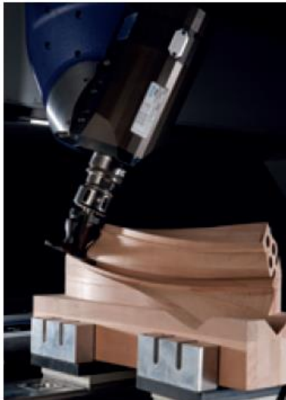
Slika 5. Homag DRIVE5C+ 5-osna radna glava ( https://www.homag.com/en/product-detail/bmg-500600_processing-centers/ )
