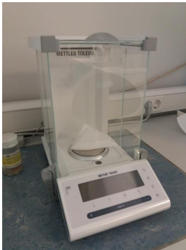
Slika 6. Vaga Mettler Toledo, NewClassic MF MS105 D4
