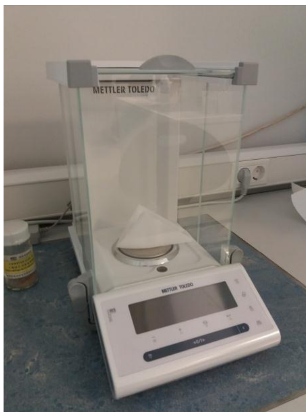
Slika 6. Vaga Mettler Toledo, NewClassic MF MS105 D4
