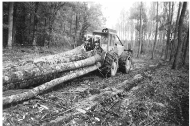
**Slika 4.** Traktor Timberjack 240C na vaci**Fig. 4** Tractor Timberjack 240C on skid trail
