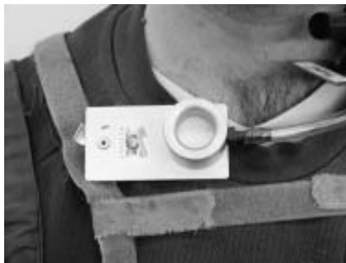
Fig. 2. Holders of filters sampling respirable particles (a) and total wood dust (b).
