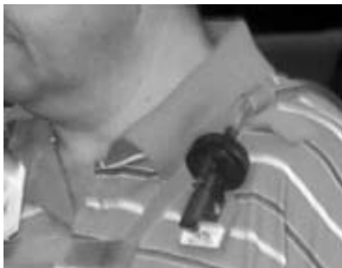
Fig. 2. Holders of filters sampling respirable particles (a) and total wood dust (b).
