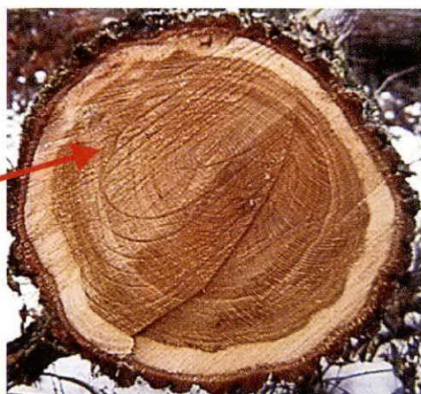
Figure 1. Cross section of oak with double sapwood zone
