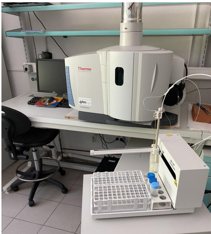
Slika 3. Instrument ICP-AES (Thermo Fisher iCAP6300 Duo)
