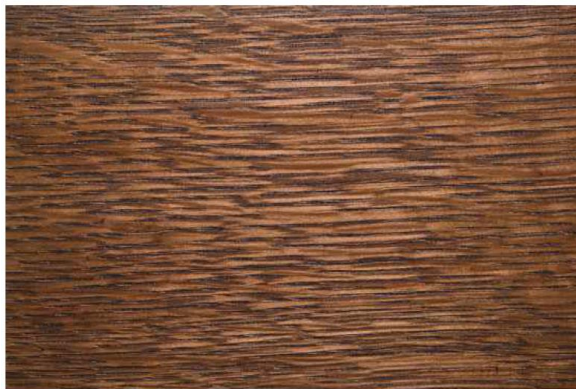
Slika 13. Uzorak hrasta nakon močenja otopinom brazilskog drva i željeznog sulfata (Miller, Crestani, 2017. The Art of Coloring Wood: A Woodworker's Guide to Understanding Dyes and Chemicals )
