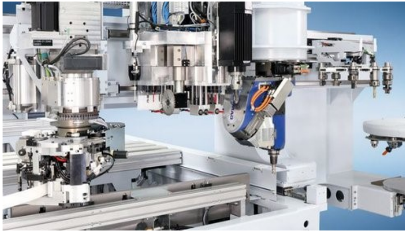
Slika 23. CNC obradni centar s agregatima za oblaganje rubova (Izvor: Vector Contour https://vectorcontour.com/blog/what-is-the-best-type-of-edge-banding-machine/ ; Pristupljeno 5.9.2022.)
