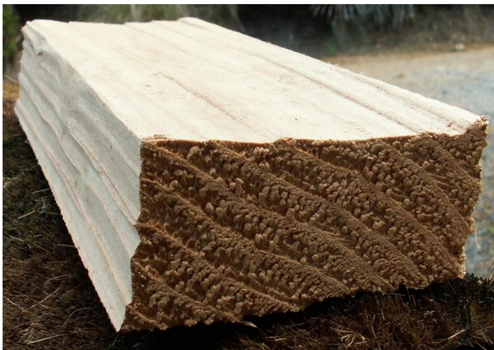
Slika 16. Prikaz kolapsa (spljoštenosti stanične stijenke) drva (izvor: https://www.nzffa.org.nz/specialty-timber-market/information-resources/sawmilling/softwoods/sawing-cedar/ , 2.7.2022.)
