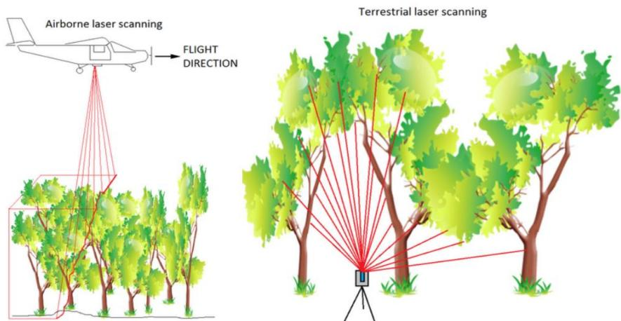
Slika 17. Razlika rada terestričkog i zračnog LiDAR-a (Izvor: AWF-WIKI [Forest Inventory Remote Sensing], 3D- Terrestrial laser scanning [http://wiki.awf.forst.uni-goettingen.de/wiki/index.php/3D\\_-Terrestrial\\_laser\\_scanning](http://wiki.awf.forst.uni-goettingen.de/wiki/index.php/3D_-Terrestrial_laser_scanning) (Pristupljeno 5.5.2023.))
