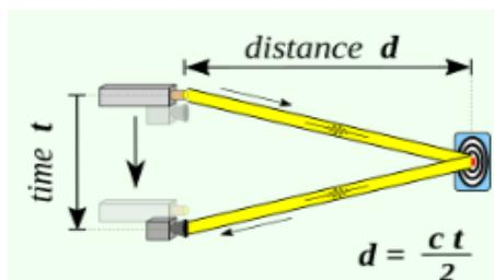
Slika 15. Način rada LiDAR-a uređaja (Izvor: Wikipedia, Time-of-flight camera [https://en.wikipedia.org/wiki/Time-of-flight\\_camera](https://en.wikipedia.org/wiki/Time-of-flight_camera) (Pristupljeno 15.4.2023.))
