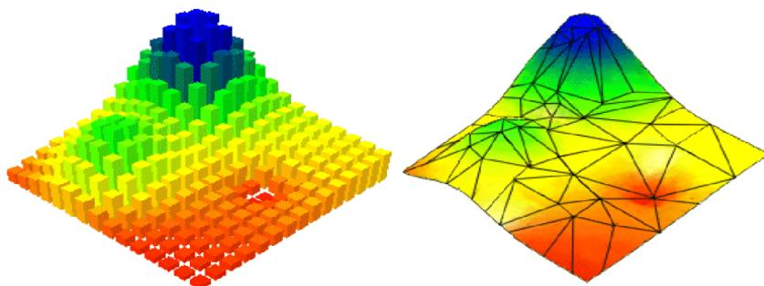
Slika 7. Usporedba GRID-a i TIN-a (Izvor: GeoComputation (David Kidner, Mark Dorey & Derek Smith), What's the point? Interpolation and extrapolation with a regular grid DEM
