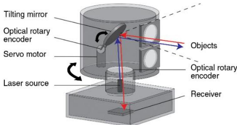
Slika 16. Dijagram LiDAR optike i kodera (Izvor: 50 RENISHAW apply inovation, Optical encoders and LiDAR scanning <https://www.renishaw.com/en/optical-encoders-and-lidar-scanning--39244> (Pristupljeno 1.5.2023.))
