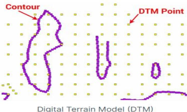
Slika 1. Prikaz Digitalnog modela reljefa pomoću slojnica (Izvor: GISGeography, DEM, DSM & DTM Differences – A Look at Elevation Models in GIS <https://gisgeography.com/dem-dsm-dtm-differences/> (Pristupljeno 5.4.2023.)
