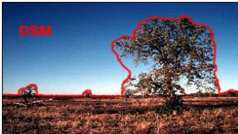
Slika 3. Prikaz Digitalnog modela površina (Izvor: GIS Resources (Saurabh Singh), Confused Between DEM, DTM and DSM! https://gisresources.com/confused-dem-dtm-dsm/ (Pristupljeno 16.4.2023.)
