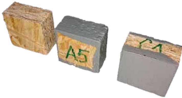
Netretirani uzorak OSB ploče i uzorci plošno i rubno tretirani epoksidnim brtvilom Untreated OSB board sample and samples with edges and surfaces treated with epoxy sealant
