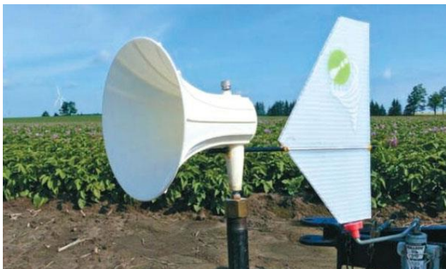
Slika 7. Pasivna klopka za spore, izvor: https://spornadosampler.com/2018/04/05/setting-the-trap-early-warnings-of-late-blight-using-passive-spore-traps/
