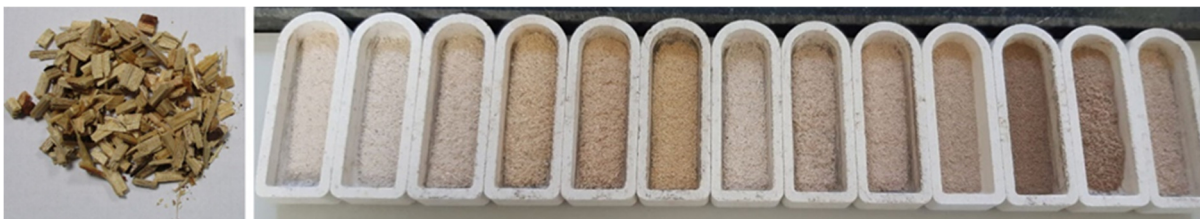
Figure 2.4. Dead wood slices from a cross-section of a wood disc (left panel) and grounded samples of dead wood prepared for analysis for carbon fraction (right panel).
