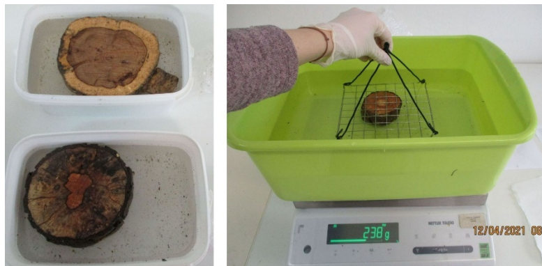
Figure 2.3. Dead wood samples immersed in the water and left there until saturation (left panel) and volume analysis of the dead wood sample using the suspension water displacement method (right panel) (Hughes 2005).
