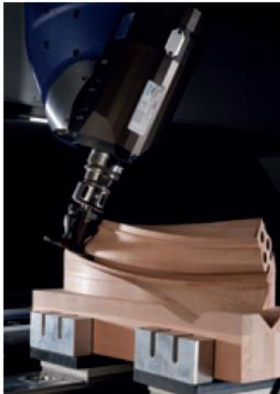
Slika 5. Homag DRIVE5C+ 5-osna radna glava ( https://www.homag.com/en/product-detail/bmg-500600_processing-centers/ )
